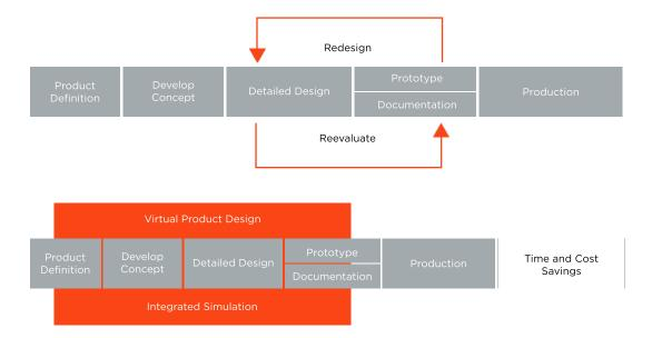
Whereas virtual product design applies integrated simulation tools across the whole design process which means that both design and process variables can be investigated together and optimized much earlier. Fewer physical prototypes, with the physical testing needed for each, significantly reduces the time and cost to market meaning fewer scrap parts, less waste, lower tooling costs, less energy while also providing confidence of fewer in-service failures.
